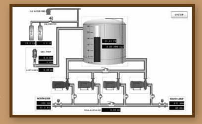
SCADA system detects there is a problem such as a High Lift Station Level. They can then connect into initiate the call out of an Operator much sooner than would have previously been possible. This enables the MUD to avoid possible spillage
